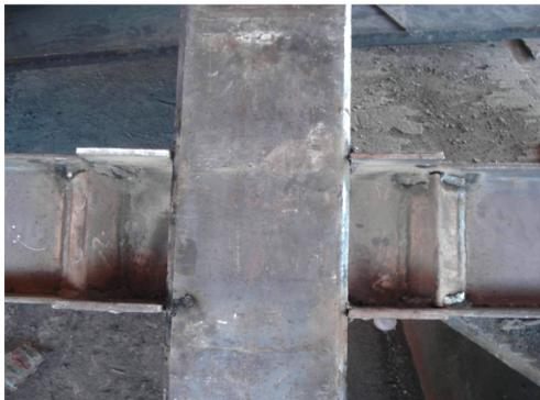
**FIGURE 2.** New RBS connection during fabrication process
